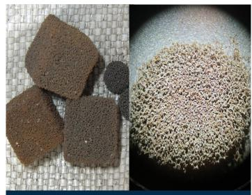
Foam-type carrier: virgin material (left) and abraded material (right).
