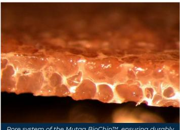
Pore system of the Mutag BioChip™, ensuring durably thin biofilms for optimal diffusion of substrate, oxygen and nutrients into all layers. Any biomass expanding out of the pores is permanently removed by shear forces.
