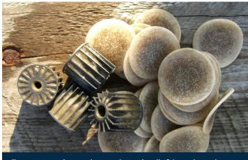
For comparison: clogged carrier (left) and unclogged carrier (right).
