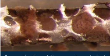
Cross section through the pore system colonized by biologically active biomass, material thickness approx. 1.1 mm.
